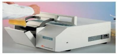
Figure 36.10 A stomacher. Paddles in this specialized blender homogenize the solid food sample in a sealed, sterile bag. The sample is suspended in a sterile solution.
