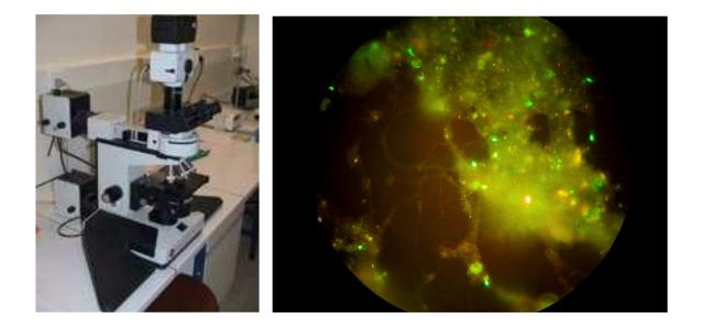
Figure 4. Epifluorescence microscope and image of a sample stained with acridine orange.
